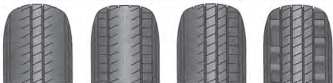
UNDER-INFLATION OVER-INFLATION POOR ALIGNMENT UNEVEN WEAR
