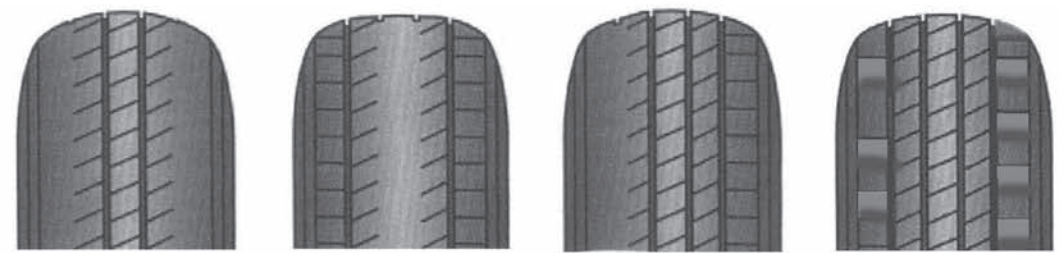
UNDER-INFLATION OVER-INFLATION POOR ALIGNMENT UNEVEN WEAR
